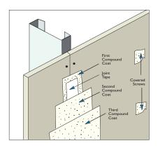
te. Use clean water to thin and mix products. Make sure temperature of the ready mix, the environment and surface of application exceed 500 F (100C) until materials are thoroughly dry and keep proper ventilation in the work area to eliminate excess moisture (Gypsum Association GA-236. We recommend the application of a drywall primer to balance the absorption of paint between the
