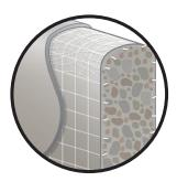
The EasyEdge strong, straight edge is wrapped with mesh embedded into the cement for extra strength. The EasyEdge ensures easy joint treatment with filler and tape, resulting in a stronger structure.
